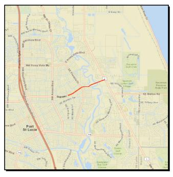
**Project Description:** Details: Right-of-way acquisition to construct bridge over St. Lucie River to connect Crosstown Parkway to US-1
