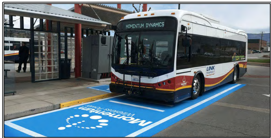
In ground inductive charging for buses - Momentum Dynamics, Lynx Transit
