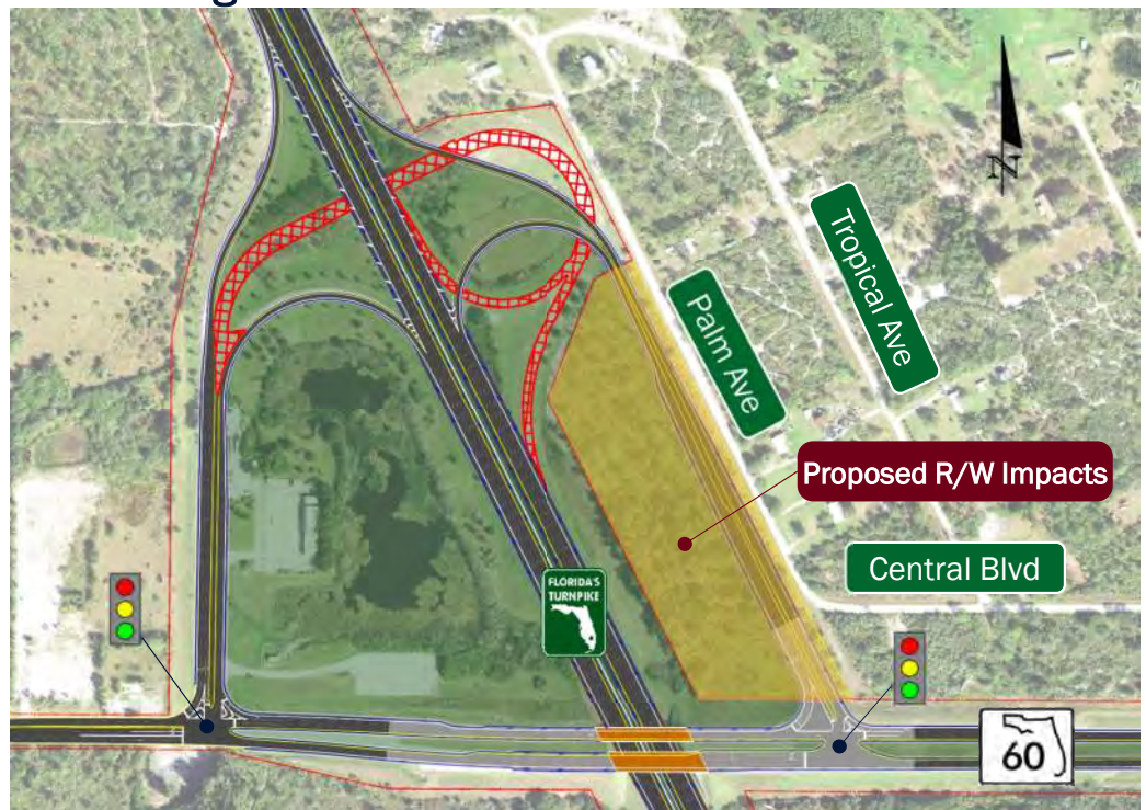
Interchange Alternative B - Partial Cloverleaf
