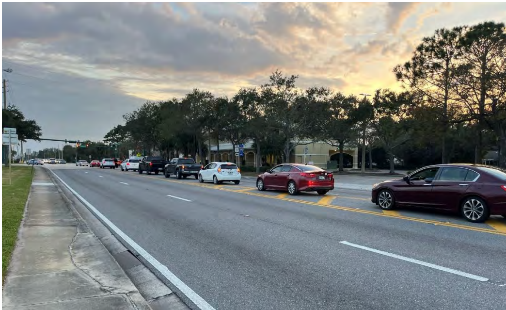
Exhibit 47: Southbound Left Turn Spillback onto Taper
