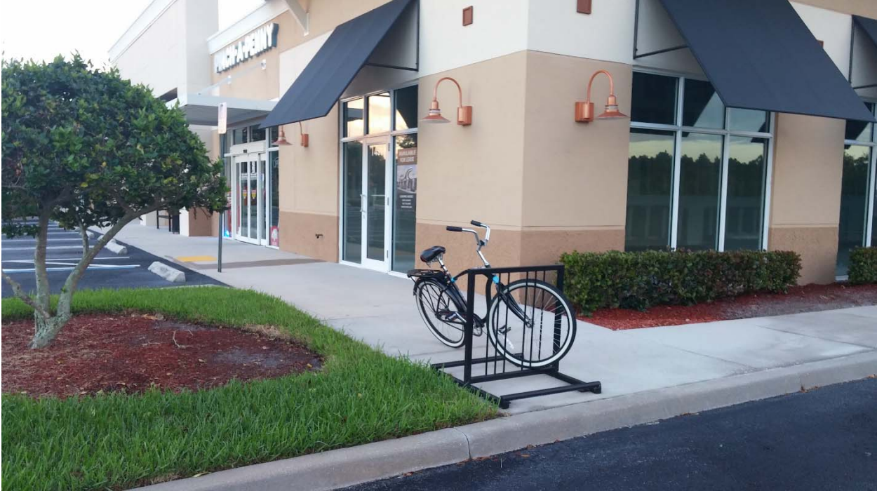
Figure 8: Near a bus stop in St Lucie West Dish Racks cause bikes to be parked like this.
