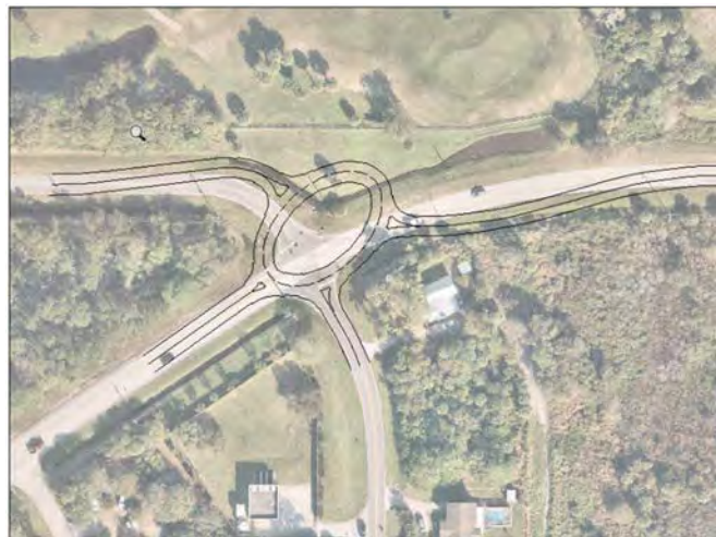
Figure 11: Single Lane Roundabout shifted North
