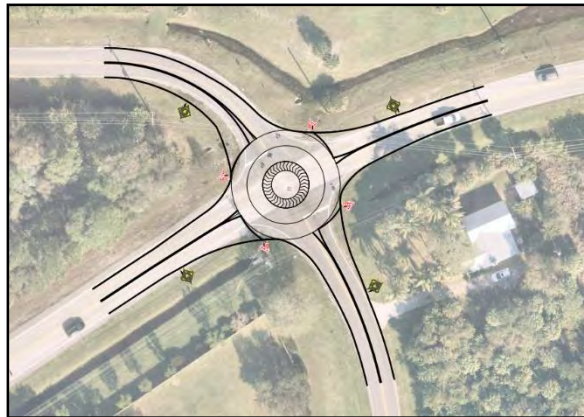
Figure 10: Single Lane Roundabout Current Location
