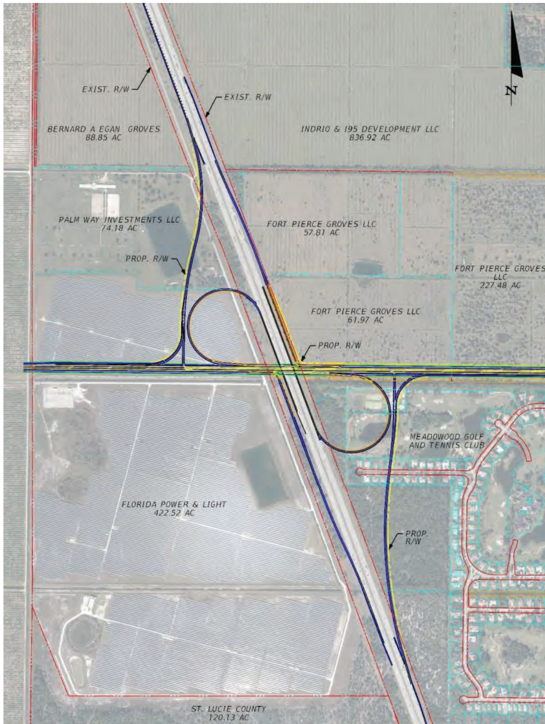
Figure 9: Northern I-95 Termini as Partial Cloverleaf Interchange
