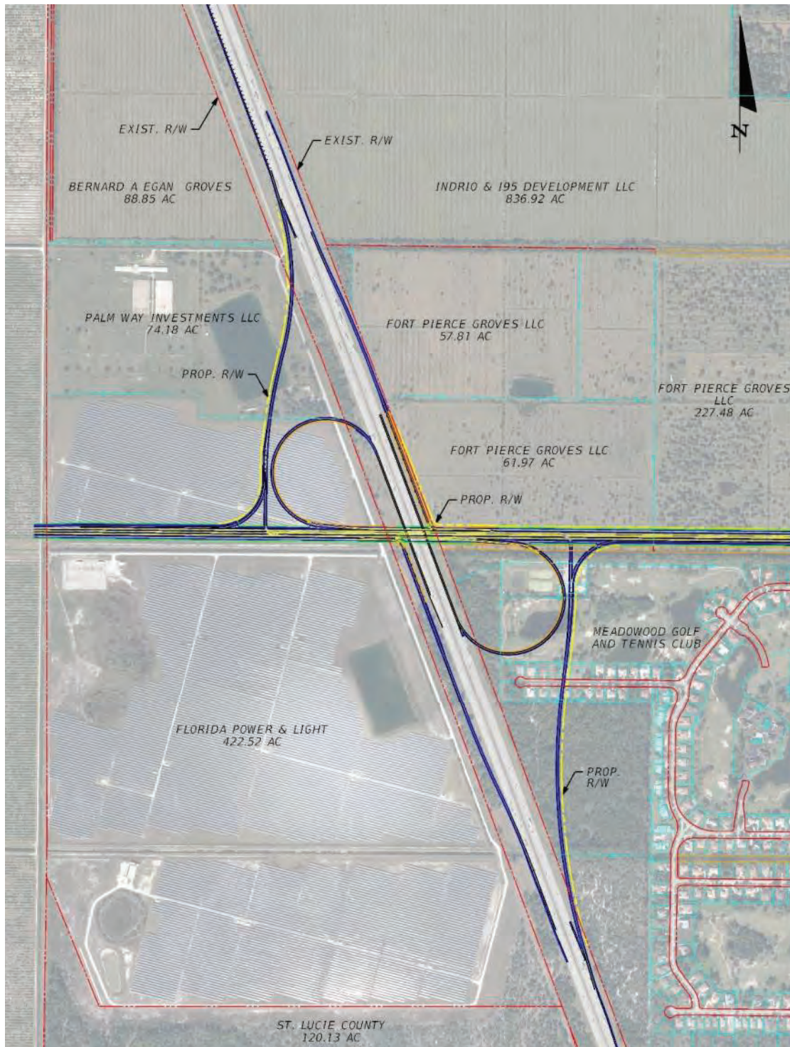
Figure 9: Northern I-95 Termini as Partial Cloverleaf Interchange
